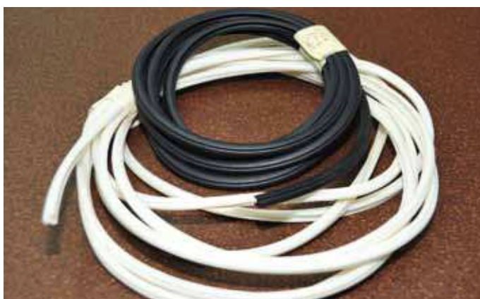
Foto 8.11 Jaluran cuaca daripada adunan getah etilena-propilena-diena-terpolimer (EPDM) dan polivinil klorida (PVC) Photo 8.11 Weather strips from ethylene-propylene-diene-terpolymer rubber (EPDM) and polyvinyl chloride (PVC) blends
