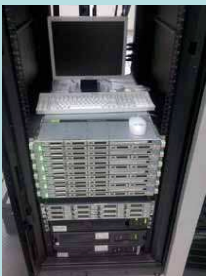
Foto 8.17 Kluster computer selari. Photo 8.17 Parallel Computer cluster
