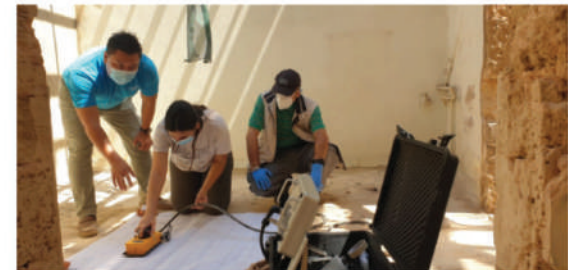
Caption Noor Azreen (left) guiding two Lebanese engineers in Beirut recently on how to perform a scanning of the floor slab using a ground penetrating radar inside a building believed to be more than a century old.
