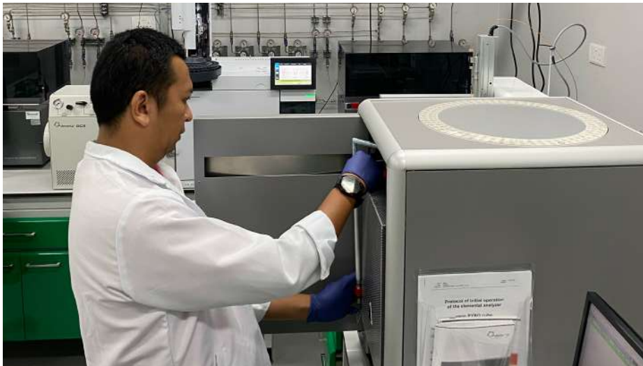
Isotope Ratio Mass Spectrometer (IRMS)
