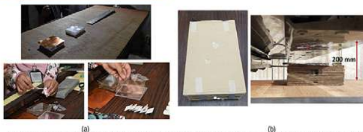
Figure 1. The setup for depth-dose profile tests (a) the assembly of polystyrene, (b) the assembly of cardboard during the irradiation.
