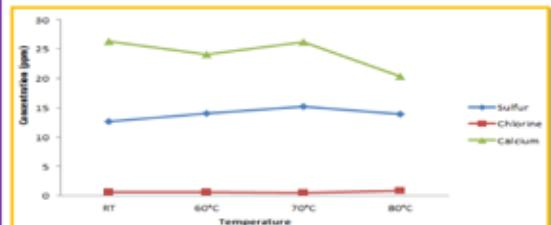
Figure 4: Concentration of inorganic element after scrubbing with different temperature of deionized water
