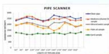
Figure 6: Graph of gamma-ray intensity profile for small pipe
