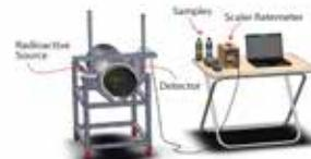
Figure 1: Schematic Diagram Experimental on Different Samples using Pipe Scanner
