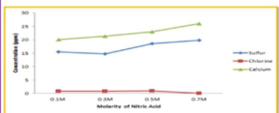
Figure 5: Concentration of inorganic element after scrubbing with different molarity of nitric acid
