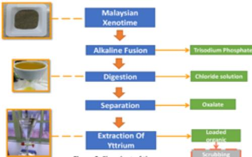
Figure 2: Flowchart of the process.
