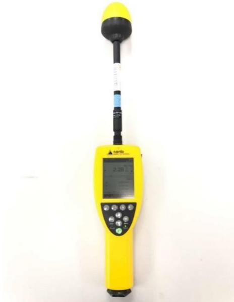
Figure 4: RF Radiation Measuring Instruments: NARDA Broadband Meter
