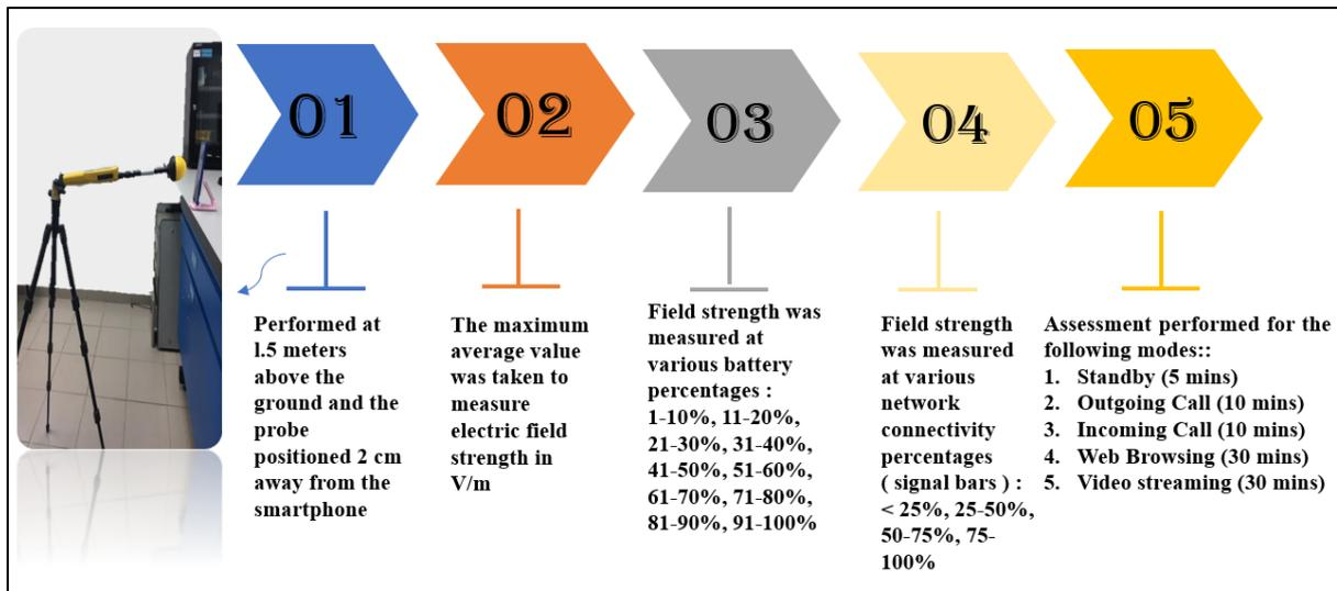
Figure 7: Summary of the steps and flow of measurement
