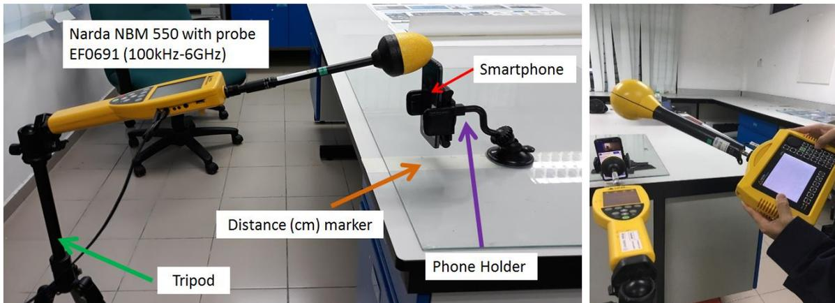
Figure 6: Equipment setup for RFR measurement (E-Field measurement)
