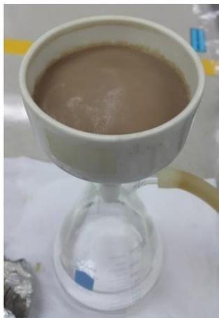
**Figure 11.** Hydrous REE oxide cake.
