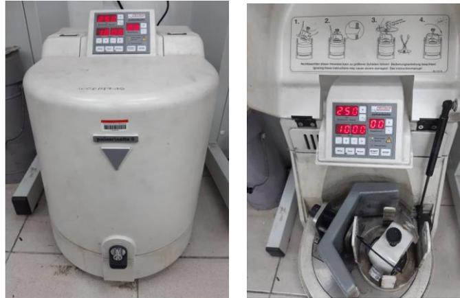
**Figure 8.** Fritsch Pulverisette ball mill.
