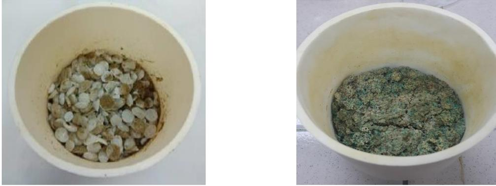
**Figure 13.** Mixture of xenotime and NaOH pellets before (left) and after (right) fusion cracking process.
