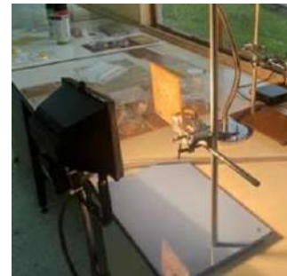
Figure 1: Experimental setup for reflection infrared thermography method.
