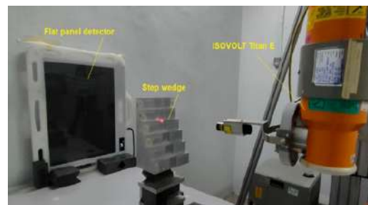
Figure 1: Experimental setup for contrast sensitivity measurement
