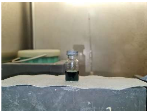
Figure 1: Irradiated chromium-51 chip when dissolved in concentrated HCL
