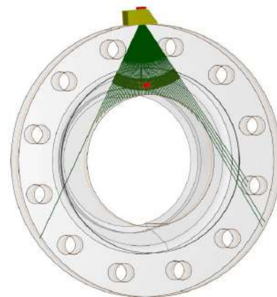
Figure 1: Model of flange inspection setup with a side drilled hole (red) and indication of beam coverage (green)
