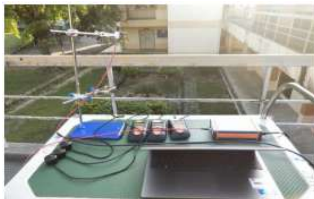
Figure 1: Set up of equipment for measuring the solar irradiation and UV Index
