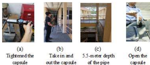
Figure 2: The experiment setup for the pressure test to the irradiation capsule
