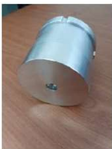
Figure 1: Faraday Cup with negative biased circuit
