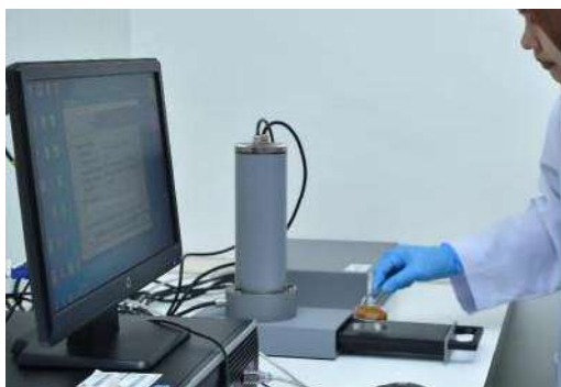
Figure 2: Analysis on detection of irradiated dried food using photostimulated luminescence
