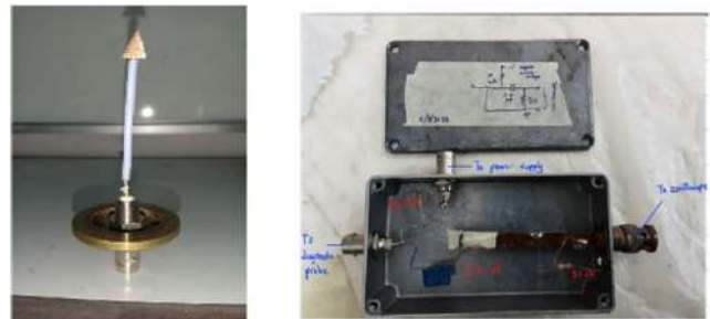
Figure 2: Ion Collector with biased circuitry
