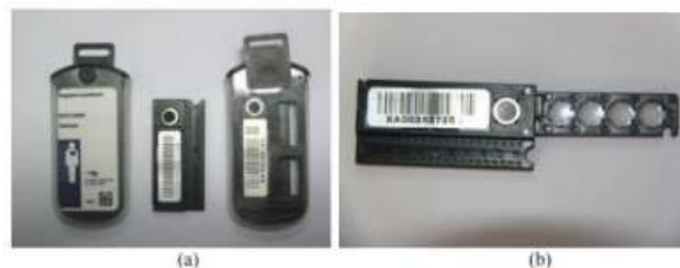
Figure 1: InLight OSLD: (a) The OSLD casing and the holders, (b) The four OSLD chips coming out from the casing.
