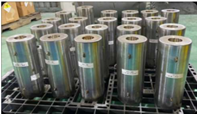
Figure 2: Waste packages for disposal in borehole.
