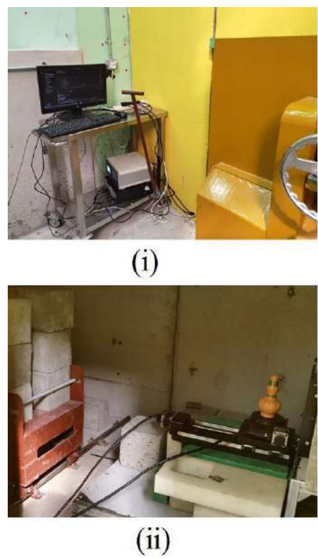
Figure 3: NuRCT system (i) control system and (ii) sample manipulator
