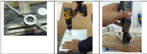
Figure 5: Die, tap and flange fabrication process
