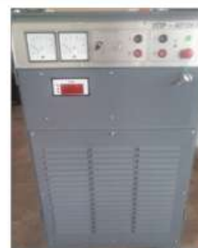
Figure 4: 50kW Direct Current Power Supply.
