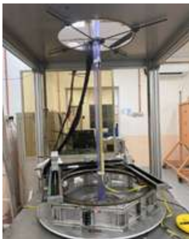
Figure 2: The gamma ray source and detector are mounted in two axial locations with motorized parallel movement.
