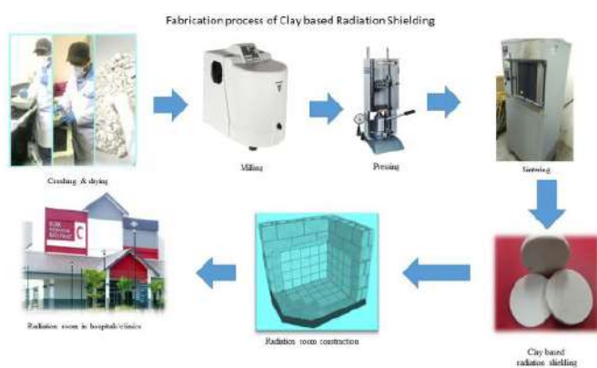
Figure 1: Fabrication process of clay based radiation shielding used dry pressing method.
