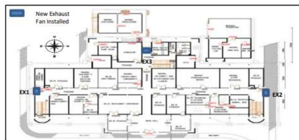
Figure 4: Layout of Block 34 with installation of 3 number of exhaust fans at suitable locations.
