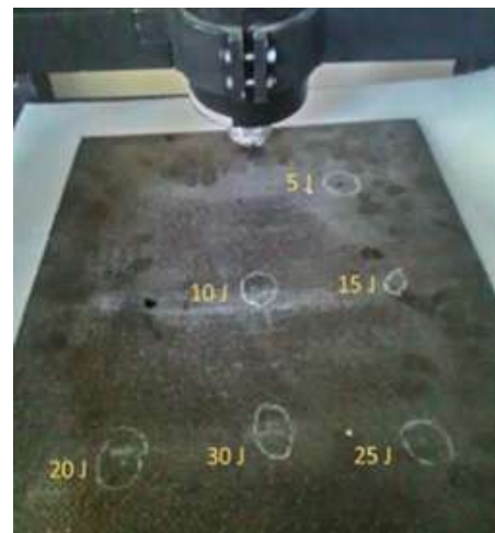
Figure 1: A 440 x 350 x 7 mm bi–directional C/C test plate with 6 locations of simulated impact damage defects.
