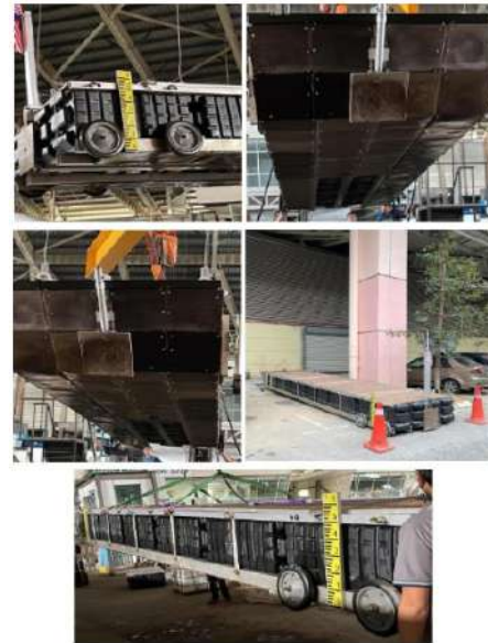
Figure 5: Structural integrity inspection post hydrodynamic test
