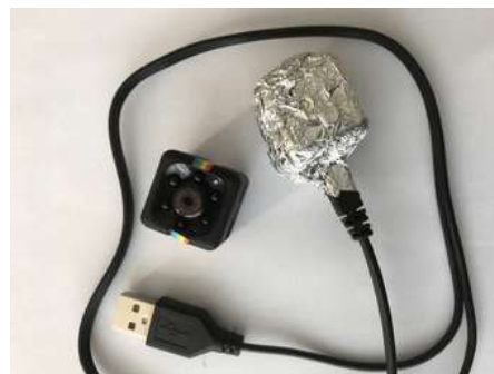
Figure 1: The webcam used for capturing ionizing events in a movie frame.
