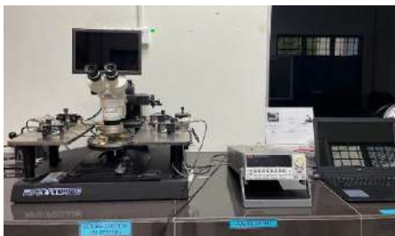
Figure 1: Full setup of probe station.
