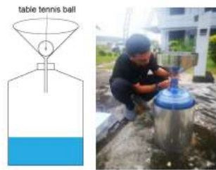
Figure 1: Precipitation Totalizer (table tennis ball) Rain Gauge Collector (IAEA, 2014)
