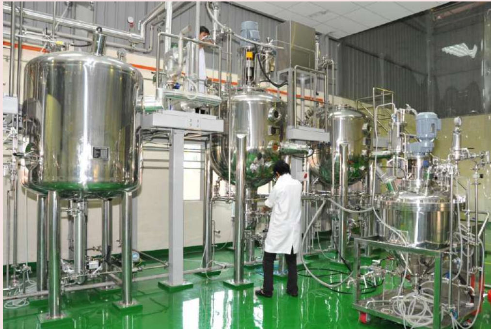
Pilot Plant of 1 ton Advanced Bioreactor System
