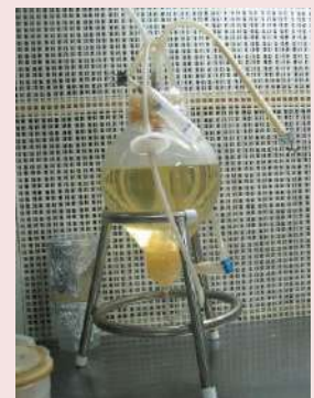
Scaling-up of cell cultures in Air-lift bioreactor
