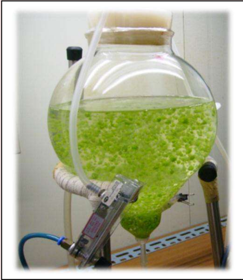
Production of somatic embryos using air-lift bioreactor
