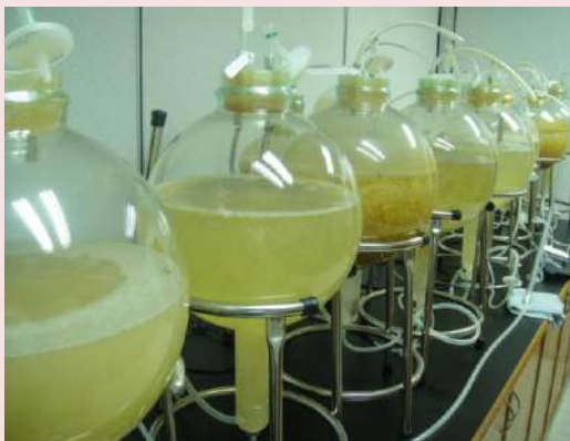
Seed-cultures in 20-litre bioreactors
