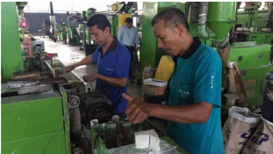
Cables such as these produced at Wonderful Ebeam Cable will be used in the engine compartment of cars. They are made heat resistant and fire retardant using irradiation.
